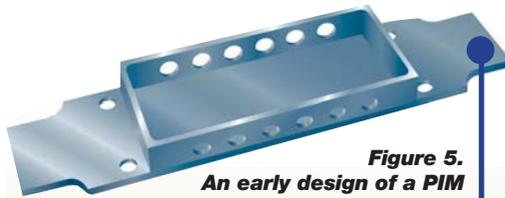
**Figure 5.** An early design of a PIM tungsten-copper package for encapsulation of microelectronic circuits. This design was successfully used in the Penn State research program to demonstrate how W-Cu composites could be produced by PIM.
